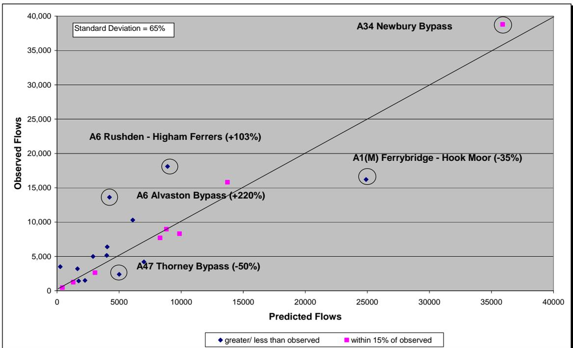
2.18 Each scheme is represented as a point (dot) on the above graph (Figure 2.1). Schemes with outturn traffic flows within a 15% threshold of the predicted flows are shown as pink dots on the graph. The blue dots are representative of old road volumes outside the 15% threshold. Schemes below the 45 degree line (drawn on the graph) have over-predicted traffic volumes and those schemes above the 45 degree line have under-predicted volumes.
